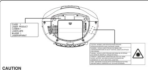
USE OF CONTROLS OR ADJUSTMENTS OR PERFORMANCE OF PROCEDURES OTHER THAN THOSE SPECIFIED HEREIN MAY RESULT IN HAZARDOUS RADIATION EXPOSURE. THIS PRODUCT SHOULD NOT BE ADJUSTED OR REPAIRED BY ANYONE EXCEPT PROP-ERLY QUALIFIED PERSONNEL.
